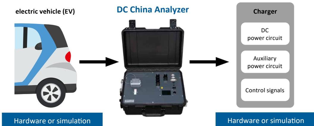
The DC China Analyzer/Simulator supports communication between electric vehicle and charger according to the standards of GB/T 27930-2011 and GB/T 27930-2015, including the support of a simplified SAE J1939-21 CAN transport protocol to handle CAN messages with a DLC up to 512 bytes.
